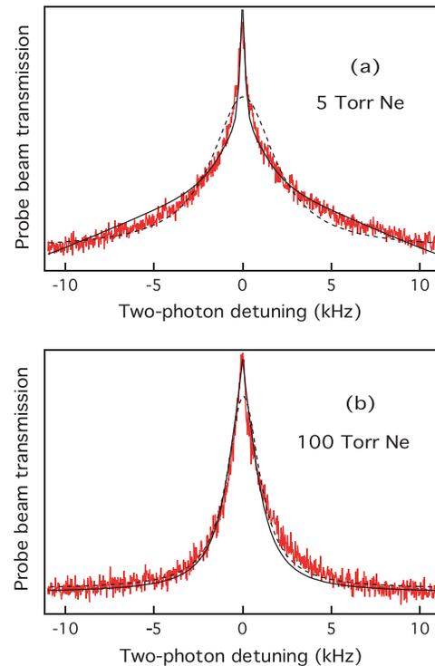
FIG. 3 (color online). Measured Rb EIT line shapes (in red) at (a) 5 and (b) 100 Torr Ne buffer gas pressure, with  $22 \mu\text{W}$  laser power and approximately 0.8 mm beam diameter. Dashed lines are fits using a Lorentzian line shape. Fitted parameters are the amplitude, off-resonant background, and full widths of approximately (a) 4.3 and (b) 2.3 kHz. Black solid lines are fits using the repeated interaction model, as described in text.
