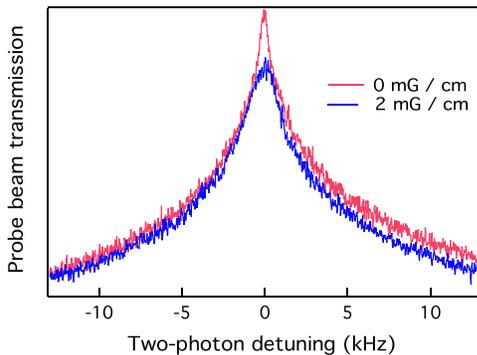
FIG. 4 (color online). Measured modification of the Rb EIT line shape by application of a transverse magnetic field gradient  $\partial B_z / \partial x = 2$  mG/cm in a 5 Torr Ne buffer gas cell with approximately 0.8 mm laser beam diameter. The field gradient suppresses the sharp peak caused by diffusion-induced Ramsey narrowing, but leaves the broader EIT line shape largely unaffected.
