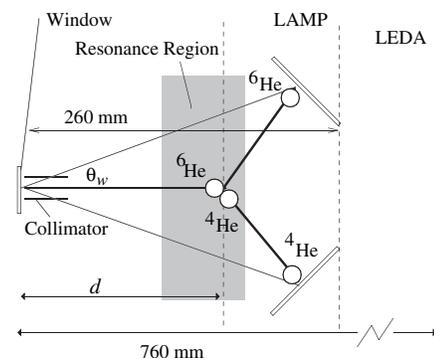
FIG. 1. Experimental setup. The region in the gas volume in which the 10.15 MeV  $^{10}\text{Be}$  resonance is formed is indicated (shaded zone). The resonance subsequently decays into  $^6\text{He} + ^4\text{He}$  which are detected in coincidence in the LAMP array.
