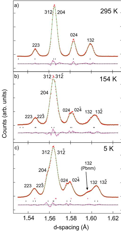
FIG. 3 (color online). Section of the diffraction pattern that shows the successive phases observed for  $\text{SmVO}_3$  with (a)  $T > T_{00}$ :  $Pbnm$  ( $R_{wp} = 0.078$ ), (b)  $T_N < T < T_{00}$ :  $P2_1/b11$  phase, (c)  $T < T_N$ :  $Pbnm$  (top markers) and  $P2_1/b11$  (bottom markers) phases ( $R_{wp} = 0.0517$ ).
