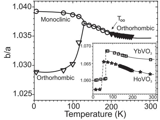
FIG. 4. Temperature dependence of the lattice parameter ratio  $b/a$  in  $\text{SmVO}_3$ : The filled triangles represent the orthorhombic phase above  $T_{00}$ . The inset presents this ratio for other  $R\text{VO}_3$  with  $R = \text{Ho}$  (stars) and  $\text{Yb}$  (squares).
