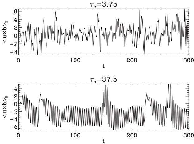
FIG. 3.  $\langle \mathbf{u} \times \mathbf{b} \rangle_x$  as a function of time for flow (10) with  $Rm = 64$ ,  $\epsilon = 0.75$ , and  $\tau_c = 3.75$  (top),  $\tau_c = 37.5$  (bottom).
