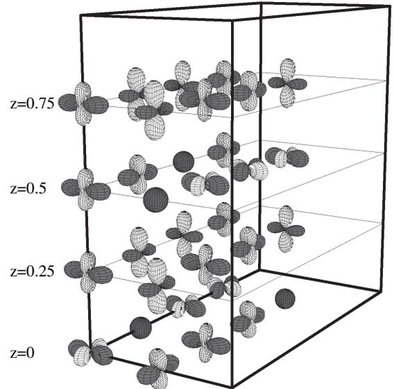
FIG. 3. Basis of the orbital polaron model for the FMI phase of  $\text{La}_{7/8}\text{Sr}_{1/8}\text{MnO}_3$  which has been used for the calculation of the structure factor. The thick solid lines indicate the  $2a_c \times 4b_c \times 4c_c$  supercell.
