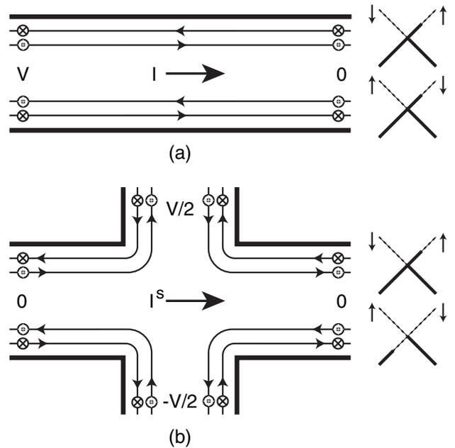
FIG. 2. Schematic diagrams showing (a) two terminal and (b) four terminal measurement geometries. In (a) a charge current  $I = (2e^2/h)V$  flows into the right lead. In (b) a spin current  $I^s = (e/4\pi)V$  flows into the right lead. The diagrams to the right indicate the population of the edge states.
