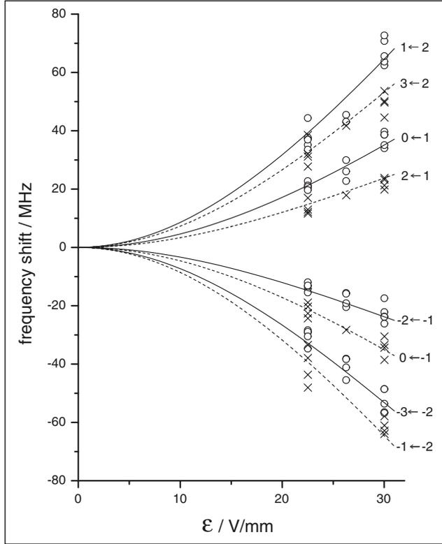
FIG. 2. Observed resonances relative to  $\nu_0$  vs electric field amplitude. The crosses indicate transitions where the direction of circular polarization was the same as that of the driving-field rotation, whereas the circles show the opposite. The  $m$  quantum transitions are indicated. The solid and dashed lines show predictions for these two cases as carried out with the aid of Eqs. (8) and (7), respectively.
