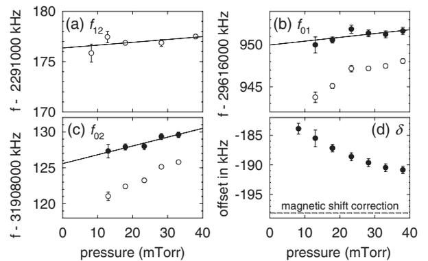
FIG. 6. Measured intervals as a function of  $^4\text{He}$  pressure  $p$  [open circles in (a)–(c)]. Offset (d) of the  $M = 0$  peak from the average of the  $M = \pm 1$  for  $P_2$  determines the light pressure shift  $\delta$ , which is then removed to get the solid dots in (b)–(c). The three intervals are then linearly extrapolated to zero  $^4\text{He}$  pressure.
