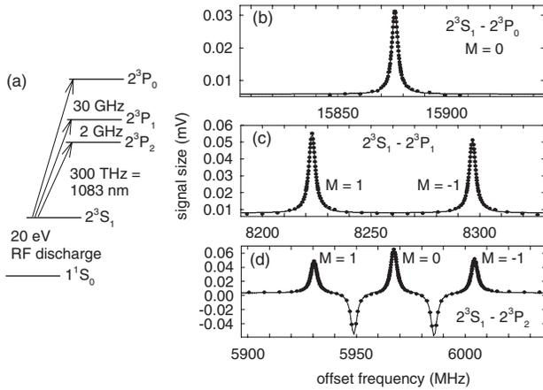
FIG. 2. Energy levels and observed transitions (arrows) are in (a), and the line shapes for each of these transitions are in (b)–(d). The probe laser transmission (points) with fits (curves) are for  $B = 52.6$  G, parallel to the pump and probe polarization axis. The two dips in (d) are crossover resonances.
