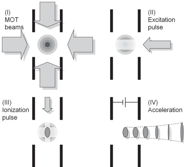
FIG. 1. Schematic of the four-step procedure to realize a pulsed UCP electron source.
