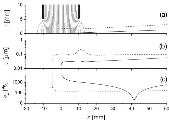
FIG. 2. (a) Field geometry and radial bunch envelope as a function of  $z$ ; (b) rms normalized emittance as a function of  $z$ ; (c) rms bunch length as a function of  $z$ . Solid lines: cigar bunch; dashed lines: pancake bunch.
