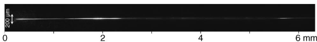
FIG. 2. Side view photograph of a filament generated in an unpumped Ti:sapphire crystal with a pulse duration of 50 fs, a focusing lens of 20 cm, and an incident energy of 3.7 mJ. The converging laser beam is incident on the left side. A filament with \sim 10 \mu\text{m} diameter is formed over the crystal length, displaying several secondary intensity maxima.
