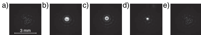
FIG. 2. Switching sequence of a solitary structure. Polarization analyzer aligned for suppression of the background beam in the detection branch: (a) background beam; (b) ignition of a soliton with circularly polarized addressing beam; (c) stable soliton with addressing beam switched off; (d) erasure of soliton with addressing beam of opposite circular polarization; (e) background beam. Parameters: mirror distance d = 120 mm; buffer gas pressure p_{N_2} = 300 mbar; cell temperature T = 321.8 °C; laser detuning \Delta = 16.2 GHz; laser power P_{\text{las}} = 219 mW; rotation of the slow axis of the eighth-wave plate with respect to input polarization \Phi = 4^\circ 30' .
