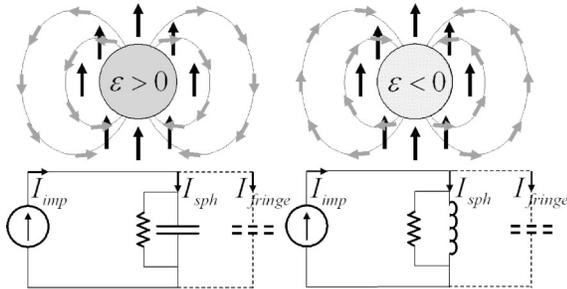
FIG. 1. A basic nanoscale circuit in the optical regime. Left: a nonplasmonic sphere with  $\varepsilon > 0$ , which provides a nanocapacitor and a nanoresistor; right: a plasmonic sphere with  $\varepsilon < 0$ , which gives a nanoinductor and a nanoresistor. Solid black arrows show the incident electric field, and the thinner field lines together with the gray arrows represent the fringe dipolar electric field from the nanosphere.
