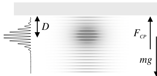
FIG. 1. Sketch of the physical situation considered in this Letter: an ultracold sample of fermionic atoms is trapped in a vertical optical lattice in proximity of a dielectric surface and performs Bloch oscillations under the combination of gravity and of the CP force.
