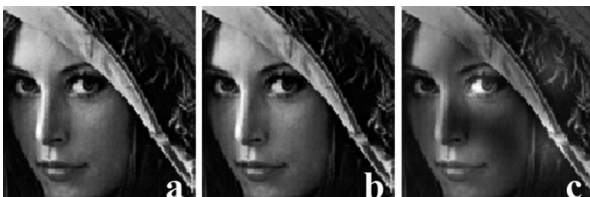
FIG. 1. Image reconstruction of oversampled diffraction patterns as a function of the number of missing waves. (a) \eta_x, \eta_y = 1 . (b) \eta_x, \eta_y = 2 . (c) \eta_x, \eta_y = 4 .
