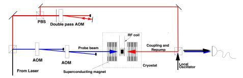
FIG. 1 (color online). The experimental setup. A beam picked of the laser was put in the remaining port of the rightmost beam splitter and is not shown. This enabled heterodyne detection of the probe beam that was transmitted through the sample.
