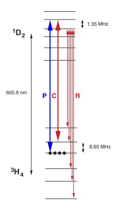
FIG. 2 (color online). Energy level diagram showing transitions driven as part of the experiment. The experiment was carried out on the zero phonon line of the  ${}^3{\rm H}_4 \rightarrow {}^1{\rm D}_2$  optical transition. The hyperfine levels are shown, and these are due to the 5/2 spin of the praseodymium nuclei. In the presence of a magnetic field these are linear combinations of the zero field states. The probe, coupling, and repump beams are labeled P, C, and R, respectively.
