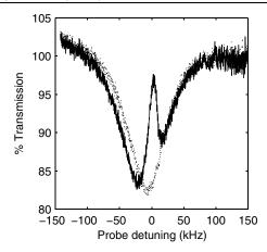
FIG. 3. Transmission of a weak probe,  $10 \mu W$ , as its frequency is swept through resonance with the prepared ensemble. The solid line was taken with a 1 mW coupling beam on and the dotted line with the coupling off.
