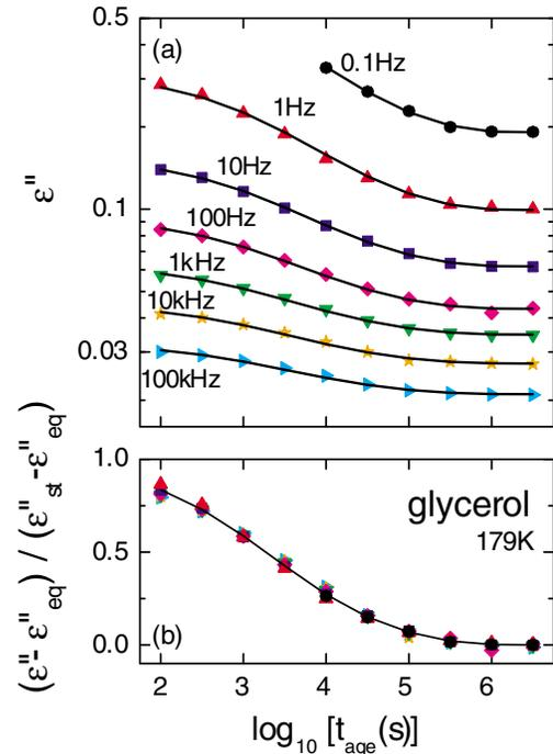
FIG. 2 (color online). (a)  $\varepsilon''(t_{\text{age}})$  of glycerol at 179 K for various frequencies. The lines are fits with the modified KWW ansatz with  $\beta_{\text{age}}$  fixed to the equilibrium value of 0.55 and identical values of  $\nu_{\text{st}}$  and  $\nu_{\text{eq}}$  for all frequencies. (b) Scaling of the curves for different frequencies, using the values of  $\varepsilon''_{\text{st}}$  and  $\varepsilon''_{\text{eq}}$  obtained from the fits shown in (a).
