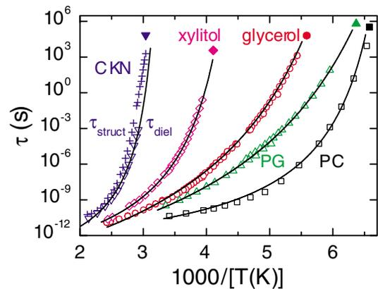
FIG. 4 (color online).  $\alpha$ -relaxation times from dielectric equilibrium measurements for the investigated glass formers (open symbols) [11,18,22,25,30]. The lines are fits with the Vogel-Fulcher-Tammann law. For CKN, in addition, the structural relaxation time from mechanical spectroscopy is plotted (pluses) [31]. The closed symbols show the equilibrium average relaxation times  $\langle \tau_{\text{eq}} \rangle$ , obtained from the fits in Figs. 2(a) and 3.
