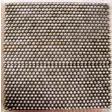
FIG. 8 (color online). fcc structure obtained by annealing with a large fracture. The plane parallel to the page is the (111) plane. The dimensions of the container are 120 mm \times 120 mm and the diameter of the beads is 4 mm.
