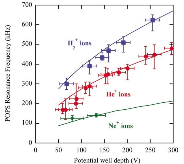
FIG. 4 (color). Comparison between the experimentally measured POPS frequencies (points) and the theoretical calculations (lines) from Eq. (3) as a function of the virtual cathode well depth and the ion mass.
