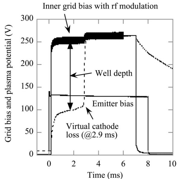
FIG. 2. HV pulse operation for the POPS oscillation measurement. Solid lines indicate the grid bias and the dotted lines indicate the plasma potential measured by the emissive probe at the center of the virtual cathode.
