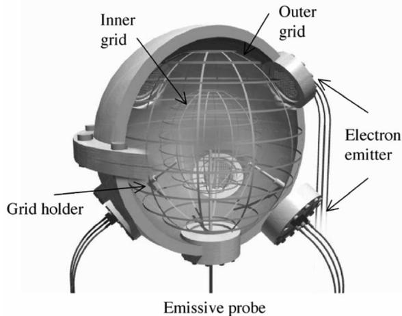
FIG. 1. Schematic of the INS-e device.
