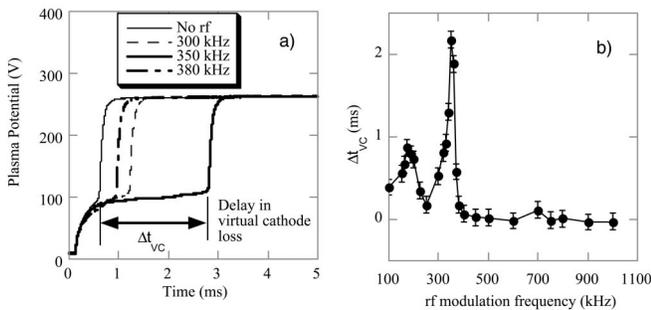
FIG. 3. (a) Temporal evolution of the plasma potential at the center of the virtual cathode with and without rf modulation. (b) Delay in the loss of the virtual cathode due to the rf modulation as a function of the modulation frequency.
