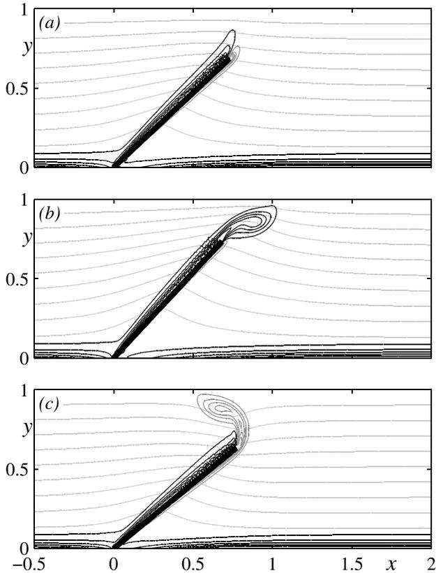
FIG. 4. Streamlines (light gray) and vorticity distribution at  $t = 0.25$ , for  $Sr = 0.1$ ,  $Re = 10^3$ , corresponding to the asymptotic curve (a) and the  $\pm 20\%$  nonasymptotic curves (b, c). Vorticity levels from  $\pm 20$  to 180 step 40; positive (clockwise) values are black, while negative values are gray.
