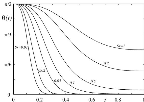
FIG. 3. Valvular opening profile for different values of the Strouhal number.
