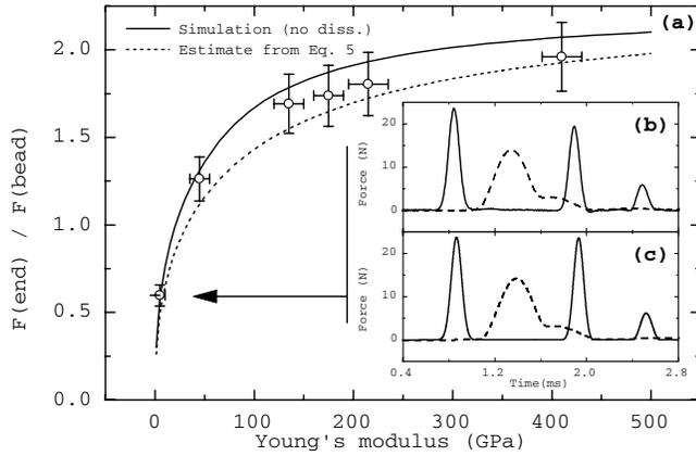
FIG. 3. (a) Ratio of force amplitudes at the end of the chain and of the incident impulse vs Young's modulus of the sample placed on the rigid sensor. Inset (b) force measurements when a solitary wave collides on the softer sample ( $Y = 5$  GPa), and (c) corresponding simulation reproducing all the experimental features for  $\eta_n = 0$ . Dashed lines indicate forces at the end of the chain. The last peaks on the right represent the secondary solitary waves.
