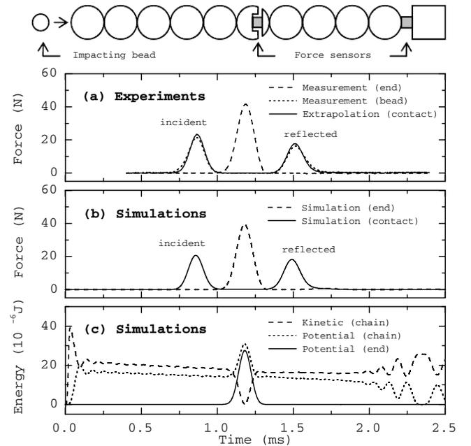
FIG. 1. (top) Schematic view of experimental setup. (a) Experiments: middle peak indicates the force signal at the end of the chain, whereas lateral peaks are the incident and reflected solitary wave. The solid line represents the force at a single contact extrapolated from Eq. (4). (b), (c) The numerical simulations of the contact forces and energy, respectively, for  $\eta_n = 2$   $\mu\text{s}$ .
