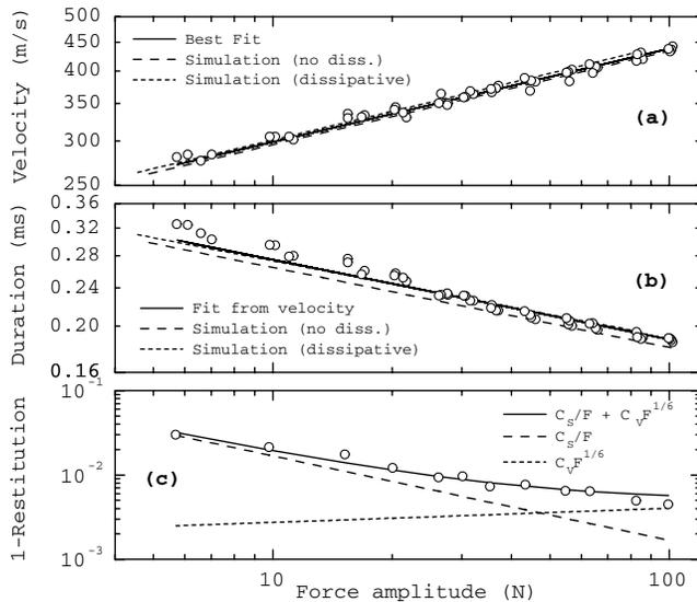
FIG. 2. (a) Velocity  $v$  and (b) duration  $2\tau$  of the solitary wave, measured inside the chain, vs force amplitude. Theoretical predictions from Eq. (3), and numerical simulations are contrasted to experimental data. (c) Restitution coefficient vs force amplitude.
