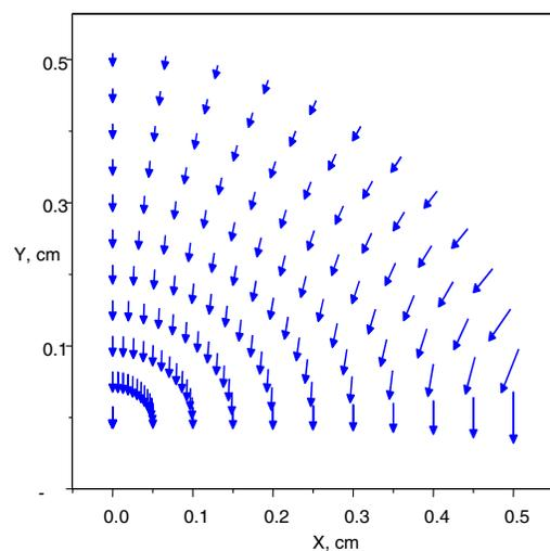
FIG. 2 (color online). Electric-field vector pattern for ideal infinite semicylindrical electrodes with a radius of 0.65 cm. Only one quadrant of the pattern is shown owing to the system symmetry. The electrode gap is along the  $x$  axis.
