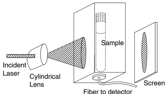
FIG. 3. Schematic of laser illumination and detection optics. For clarity of presentation, the electrodes, which are inside the insulated box that surrounds the sample, are not shown in this diagram.
