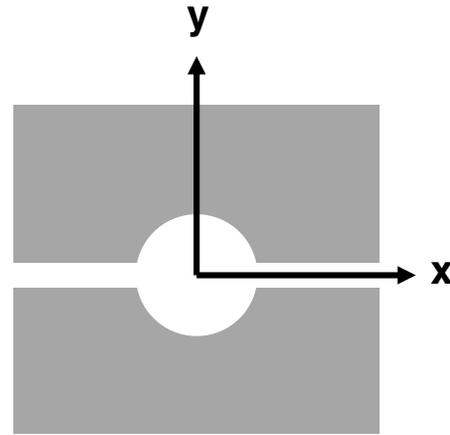
FIG. 1. Cross section of brass electrode assembly. Gap spacing is not to scale in this schematic drawing. All sharp edges were rounded in the actual electrodes.
