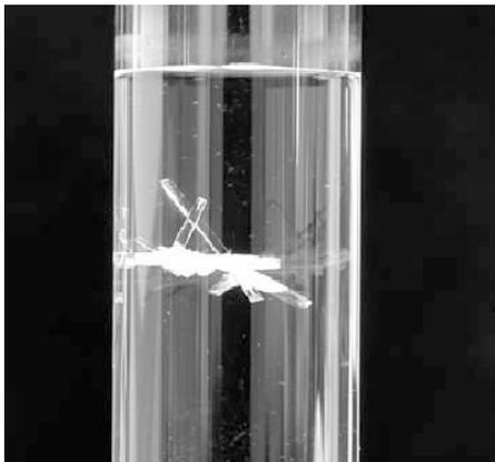
FIG. 4.  $\gamma$ -glycine crystals formed by dc-electric-field-induced nucleation.
