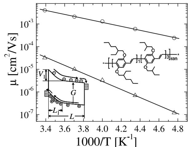
FIG. 1. Experimental charge carrier mobility of the electrons ( $\mu_e$ ,  $\circ$ ) and holes ( $\mu_h$ ,  $\triangle$ ) as a function of temperature  $T$ . The  $\mu_e$  and  $\mu_h$  have been determined from space-charge limited measurements on 20:80 blends of BEH<sub>1</sub>BMB<sub>3</sub>-PPV:PCBM. The inset schematically shows a photovoltaic device under illumination and the chemical structure of the BEH<sub>1</sub>BMB<sub>3</sub>-PPV, respectively.
