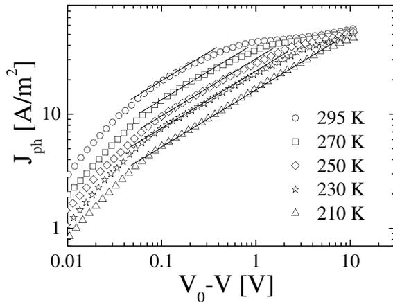
FIG. 2. Temperature dependence of the photocurrent (symbols) in a 20:80 blend of BEH<sub>1</sub>BMB<sub>3</sub>-PPV:PCBM versus effective applied voltage ( $V_0 - V$ ) for a device of 275 nm thickness illuminated at an intensity of 80 mW/cm<sup>2</sup>. The solid lines represent the square-root dependence of the photocurrent  $J_{ph}$  on effective voltage, used here as a guide for the eye.
