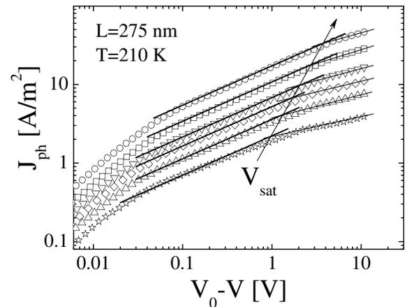
FIG. 3. Incident light power (ILP) dependence of the photocurrent ( $J_{ph}$ ) versus the effective voltage ( $V_0 - V$ ) measured at  $T = 210$  K. The solid (thick) lines represent the calculated  $J_{ph}$  from Eq. (4) using  $\mu_h = 1.2 \times 10^{-7}$  cm<sup>2</sup>/V s,  $\epsilon_r = 2.6$ , and  $G \propto \text{ILP}$ , where ILP was varied from 80 to 6 mW/cm<sup>2</sup>. The arrow indicates the voltage ( $V_{sat}$ ) at which  $J_{ph}$  shows the transition to the saturation regime.
