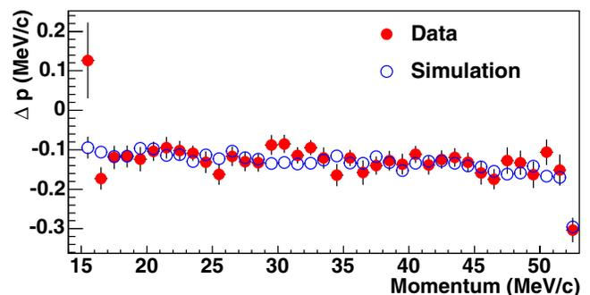
FIG. 2 (color online). Average momentum change of decay positrons through the target and detector materials as a function of momentum for data (solid circles) and Monte Carlo simulations (open circles), measured as described in the text.
