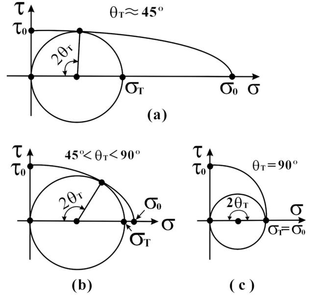
FIG. 2. Schematic illustration of the ellipse criterion at different conditions: (a)  $\alpha = \tau_0/\sigma_0 \rightarrow 0$  or  $\sigma_0 \rightarrow \infty$  and  $\theta_T \approx 45^\circ$ ; (b)  $0 < \alpha = \tau_0/\sigma_0 < \sqrt{2}/2$  and  $45^\circ < \theta_T < 90^\circ$ ; (c)  $\alpha = \tau_0/\sigma_0 \geq \sqrt{2}/2$  and  $\theta_T = 90^\circ$ .
