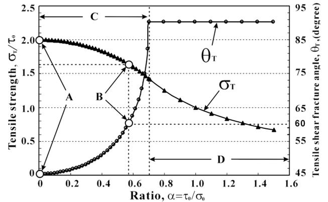
FIG. 3. Dependence of tensile fracture strength  $\sigma_T$  and tensile shear fracture angle  $\theta_T$  on the ratio  $\alpha = \tau_0/\sigma_0$  according to the ellipse criterion. In a different range of  $\alpha = \tau_0/\sigma_0$ , each of the four classical failure criteria can be unified by the present ellipse criterion.
