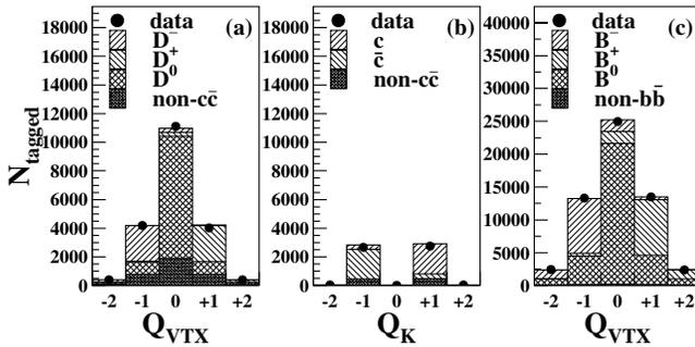
FIG. 2. Distributions of hemisphere charge: (a)  $Q_{V_{TX}}$ ,  $y_{\text{hem}} < 0.4$ ; (b)  $Q_K$ ,  $y_{\text{hem}} < 0.4$  (the large  $Q_K = 0$  contribution is suppressed); (c)  $Q_{V_{TX}}$ ,  $y_{\text{hem}} > 0.85$ , including VXD-only tracks. The  $D^+$ ,  $D^-$ ,  $D^0$ , and  $B^+$ ,  $B^-$ ,  $B^0$  designations refer to all positive, negative, or neutral heavy flavor hadrons, including baryons, from the MC simulation.
