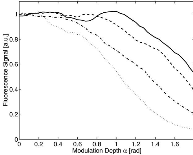
FIG. 3. TPA measurement for spectral phase function of  $\Phi(\omega) = \alpha \sin(\beta(\omega - \omega_0/2) + \pi/4)$  for which  $\varepsilon^2(t)$  has an imaginary part. The TPA is measured as a function of the modulation depth  $\alpha$  for pulse intensities (at the center of the beam) of  $0.1I_{\max}$  (dotted line),  $0.5I_{\max}$  (dashed-dotted line),  $0.8I_{\max}$  (dashed line) and  $I_{\max}$  (solid line).
