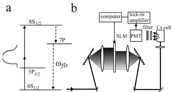
FIG. 1. (a) Energy level diagram of the two-photon transition  $6S \rightarrow 8S$  in atomic Cs. Wavelengths longer than 840 nm are blocked as they spectrally overlap the  $5P_{3/2}$  level. (b) Outline of the experimental setup.
