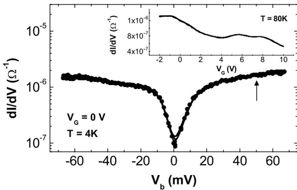
FIG. 1. Differential conductance vs applied bias voltage at 4 K for  $V_G = 0$  V. The arrow indicates the high energy regime studied under 50 T at 4 K. In the inset, the gate voltage effects on the differential conductance for  $V_b = 20$  mV at 80 K.
