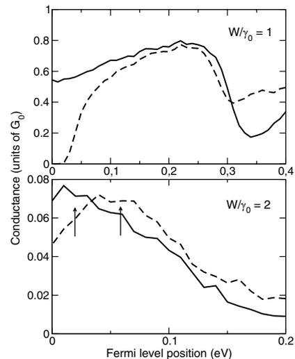
FIG. 4. Conductance versus Fermi level position, for a disordered (22, 22) nanotube, and two values of the parallel magnetic field:  $B_{\parallel} = 0$  T (solid line) and  $B_{\parallel} = 50$  T (dashed line). Two disorder strengths are considered:  $W/\gamma_0 = 1$  (upper panel) and  $W/\gamma_0 = 2$  (lower panel). In the strong disorder case, the two arrows indicate possible Fermi level positions for  $V_G = 0$  V (left) and  $V_G = 10$  V (right).
