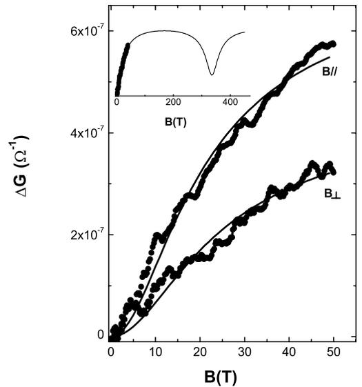
FIG. 2. Magnetoconductance  $\Delta G(B)$  up to 50 T for  $B_{\parallel}$  and  $B_{\perp}$  with a bias voltage  $V_b = 300$  mV and zero gate voltage at 80 K. Solid lines represent the quasi-2D WL fits for both configurations. Inset: the predicted  $\Delta G(B_{\parallel})$  from Eq. (1) in a very high field, superimposed to our measurement.
