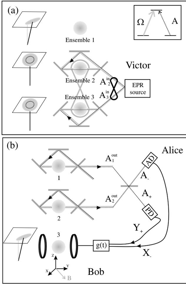
FIG. 1. Teleportation scheme: (a) *Preparation*. Insert:  $\Lambda$ -type level structure considered. Left: schematic atomic initial states for each ensemble (for spins 2 and 3, the dashed circle indicates the coherent spin state fluctuation distribution). (b) *Measurement and reconstruction*. Left: teleported state after reconstruction is completed. AD: amplitude detector. PD: phase detector.
