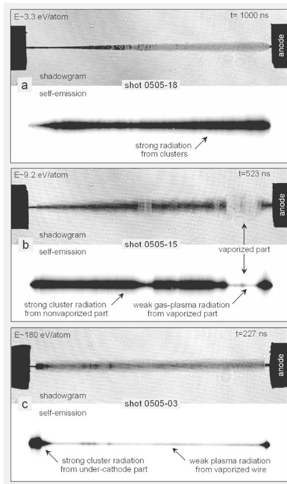
FIG. 1. Three complimentary sets of laser shadowgrams (top) and time-integrated self-emission images (bottom) of exploding 12  $\mu\text{m}$  diameter and 2 cm long W wires with different values of deposited energy: (a) fast explosion of bare wire at 1000 ns; (b) slow explosion of coated wire at 523 ns; (c) fast explosion of coated wire at 227 ns.
