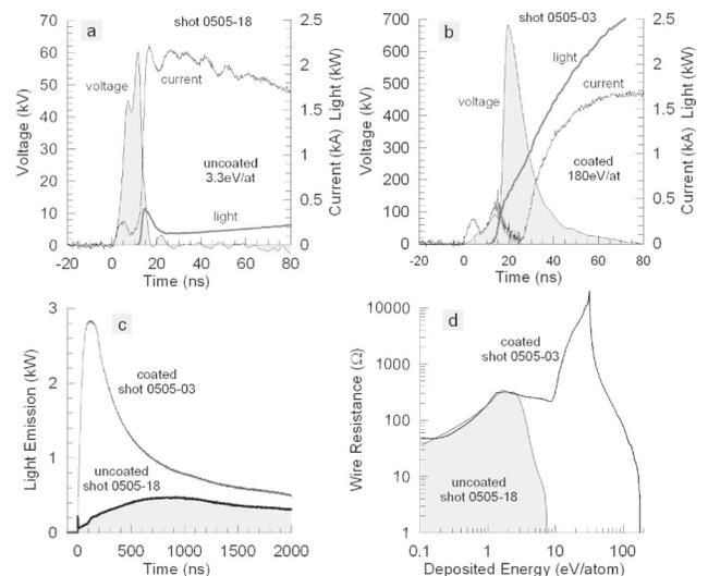
FIG. 2. Waveforms for current, voltage, and light emission for fast-exploding 12  $\mu\text{m}$  W wires: (a) bare and (b) coated. (c) Dependence of long-time behavior of white-light emission for coated and bare wires. (d) Dependence of wire resistance on deposited energy for coated and bare wires.
