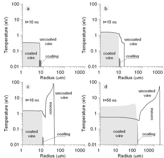
FIG. 3. Radial temperature profiles at different moments of time for explosion in vacuum of bare (line) and coated (shaded) 12  $\mu\text{m}$  diameter W wires. The coating itself is indicated by darker shading.
