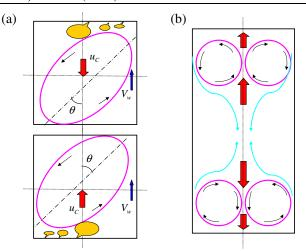
FIG. 6 (color online). (a) Elliptical flow pattern of  $\Gamma = 1$  which departs from the *z* axis with an angle of  $\theta$ . When bottom (top) plumes are active, upward (downward) velocity  $u_c$  is observed at the cell center.  $V_w$  is the mean velocity at the sidewall. (b) Flow pattern of  $\Gamma = 0.5$ . Axisymmetric toroidal rings exist steadily near the upper and lower plates. The mean velocity direction on the *z* axis is indicated by thick arrows.
