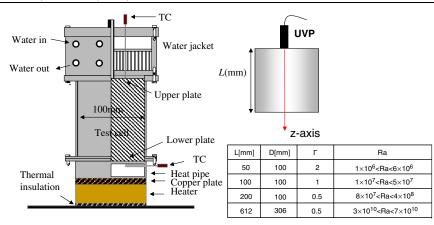
FIG. 1 (color online). Schematic view of experimental apparatus and coordinate system.
