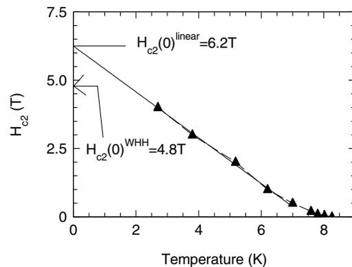
FIG. 6.  $H_{c2}(T)$  plot defined by the onset temperature of the resistive transition measured in magnetic fields for the  $\text{Li}_2\text{Pd}_3\text{B}$  sample.
