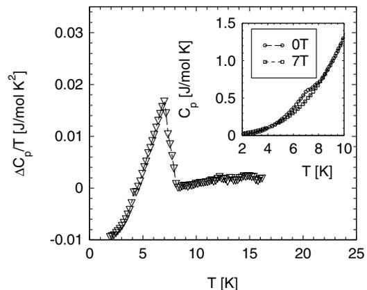
FIG. 2.  $\Delta C_p/T$  plotted as a function of temperature, where  $\Delta C = C_p(0 \text{ T}) - C_p(7 \text{ T})$ . The inset shows the experimental curves of specific heat  $C_p(0 \text{ T})$  and  $C_p(7 \text{ T})$  as a function of temperature measured in the zero applied magnetic field and 7 T, respectively.
