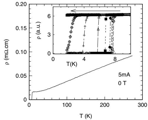
FIG. 5. Temperature-dependent resistivity measured for the  $\text{Li}_2\text{Pd}_3\text{B}$  bulk sample (a few mm size). The inset shows the resistivity transitions in applied magnetic fields  $H$  of 0, 0.05, 0.1, 0.2, 0.5, 1, 2, 3, 4, and 5 T (the arrow indicates the increase in  $H$ ). The applied current was 5 mA for a 4-probe configuration.
