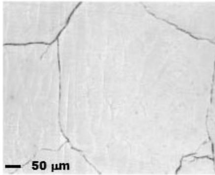
FIG. 3. Optical microstructure on the cross section of the arc-melted  $\text{Li}_2\text{Pd}_3\text{B}$  button.
