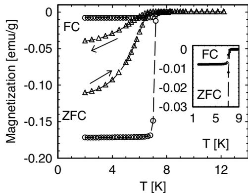
FIG. 1. Magnetization vs temperature curves for the  $\text{Li}_2\text{Pd}_3\text{B}$  sample measured in zero-field-cooling (ZFC) and field-cooling (FC) arrangements in the magnetic field of 20 Oe: circles, arc-melted bulk sample, and triangles, powdered sample. The inset shows in detail the FC curve of the arc-melted bulk sample.
