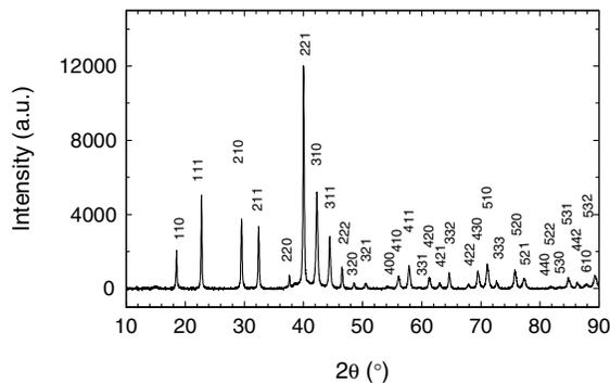
FIG. 4. XRD powder pattern of the  $\text{Li}_2\text{Pd}_3\text{B}$  sample synthesized by arc melting.
