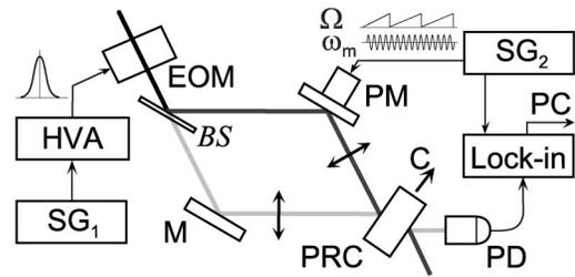
FIG. 2. Schematic of the experimental setup with photorefractive crystal (PRC), electro-optic modulator (EOM), beam splitter (BS), mirror (M), piezoelectrically driven mirror (PM), photodiode (PD), signal generators (SG1 and SG2), high voltage amplifier (HVA), and lock-in amplifier. The arrow near the sample indicates the positive direction of the spontaneous polarization; double arrows show the polarization of the light waves.
