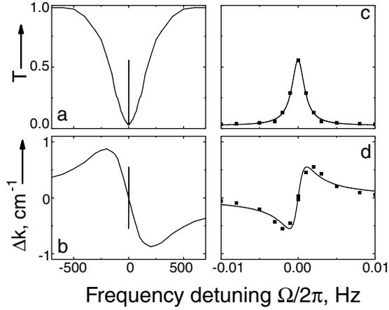
FIG. 3. Experimental dependences of sample transmission  $T$  (a),(c) and variation of propagation constant  $\Delta k$  (b),(d) of a weak signal wave on frequency detuning of the signal wave.
