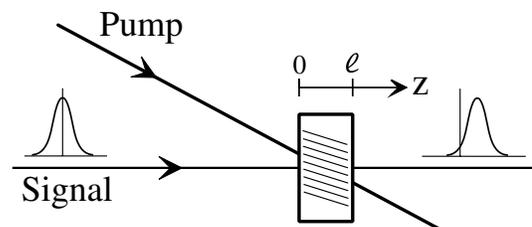
FIG. 1. Schematic of pulse propagation through a photorefractive crystal in the presence of a coherent pump wave.
