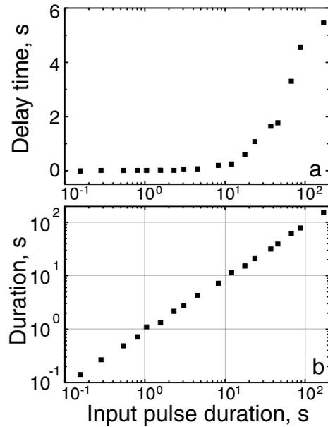
FIG. 4. Time delay of the output pulse maximum (a) and output pulse duration (b) as a function of input pulse duration;  $I_p = 1$   $\text{W/cm}^2$ , grating spacing  $\Lambda = 1.8$   $\mu\text{m}$ .
