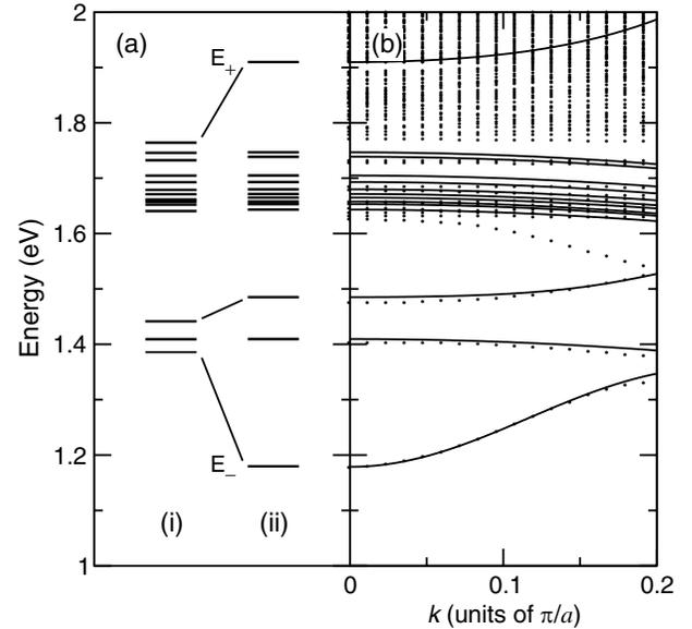
FIG. 1. (a) Calculated N cluster-state energies  $\varepsilon_l$  and CBE energy in a  $\text{Ga}_{500}\text{N}_{13}\text{As}_{487}$  supercell (i) before and (ii) after inclusion of interaction with CBE. (b) Supercell band dispersion obtained by TB (dots) and LCINS methods (solid lines).
