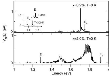
FIG. 2. Calculated distribution of  $N$  cluster-state energies  $\varepsilon_l$  weighted by the square of their interactions  $|V_l|^2$  with the CBE state for  $\text{GaN}_{0.002}\text{As}_{0.998}$  and for  $\text{GaN}_{0.02}\text{As}_{0.98}$ . Inset: expanded view of the  $N$  pair state spectrum relative to the  $E_-$  level for  $x = 0.2\%$  at  $T = 0$  K and  $T = 300$  K.
