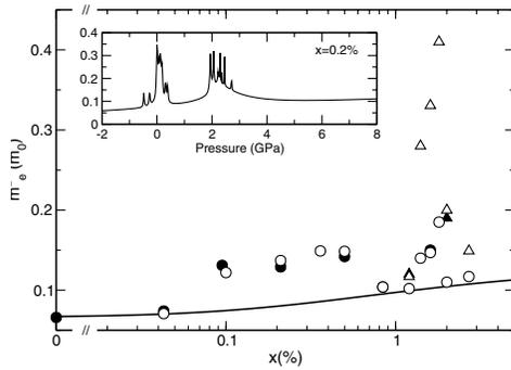
FIG. 4. Solid data points: measured low temperature electron effective mass  $m_e^*$  in bulk (circles) and quantum well (triangles) samples. Open symbols (solid line):  $m_e^*$  calculated using LCINS (BAC) method. Inset: calculated variation of  $m_e^*$  with pressure in a bulk  $\text{GaN}_{0.002}\text{As}_{0.998}$  epilayer at  $T = 0$  K.
