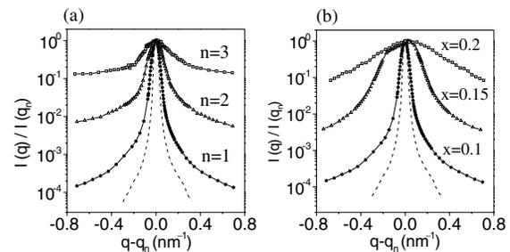
FIG. 2. X-ray line shape of elastomer II; the dashed line gives the direct beam. (a) Three orders of diffraction peaks for crosslinks density  $x = 0.1$ . (b) First-order peak for  $x = 0.1, 0.15$ , and  $0.2$ , respectively.
