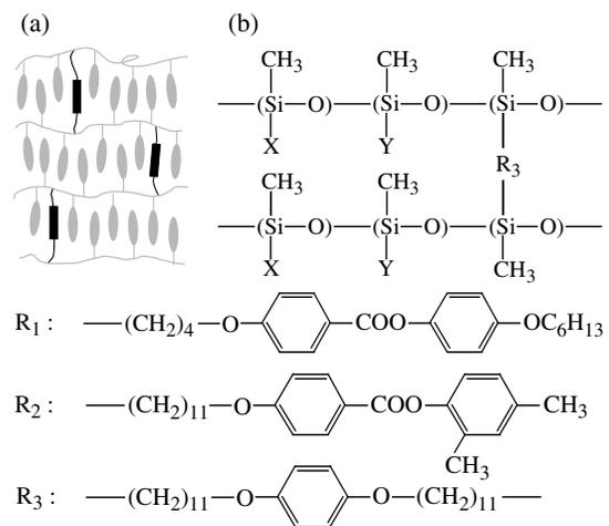
FIG. 1. (a) Schematic picture of smectic elastomers. (b) Chemical structures. Elastomer type I has  $X = Y = R_1$ ; type II has  $X = R_1$  (45%) and  $Y = R_2$  (55%).
