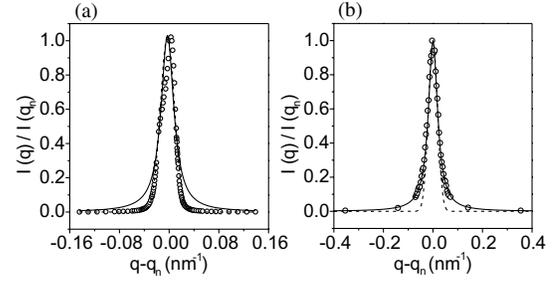
FIG. 3. First harmonic line shape of elastomer II for (a) crosslink density  $x = 0.15$ , and (b)  $x = 0.2$ . The dashed line is the best fit to a Gaussian, the full line to a Lorentzian.
