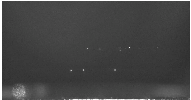
FIG. 1. Particles 3.42 \mu\text{m} shortly after the injection in the plasma. P = 46 Pa and electrode excitation V_{RFpp} = 300 V. The picture shows 17 \times 8.8 mm.
