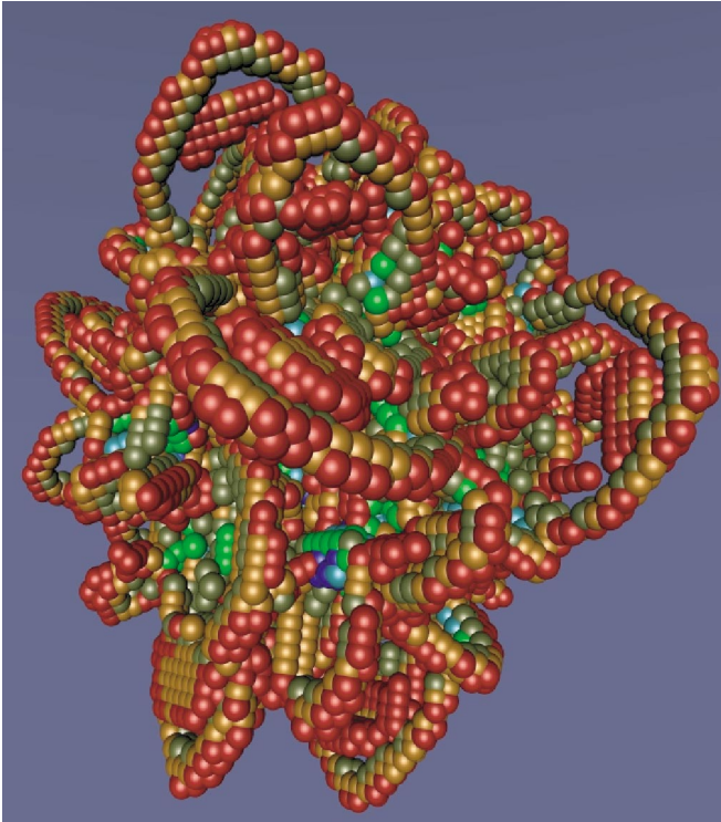
FIG. 5 (color). Final detachment of the \frac{1}{2}\langle 110 \rangle \{001\} dislocations corresponding to a dilatation of 34.5%.
