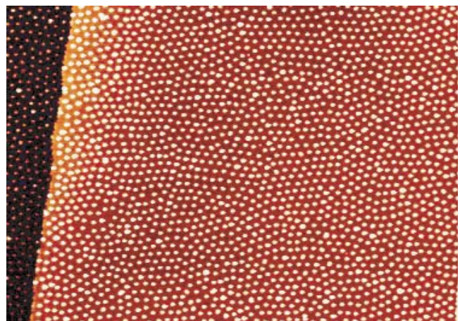
FIG. 1 (color online). Constant current STM image ( 155 \times 108 nm 2 , V_S = -90 mV, I = 40 pA) of approximately 1% ML Ce with d = 3.2 nm on a Ag(111) surface at 3.9 K. Dark (bright) contrast: lower (upper) terrace separated by a monatomic Ag step.
