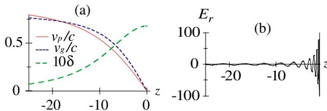
FIG. 2 (color). (a) Phase velocity  $v_p$ , group velocity  $v_g$ , and adiabatic parameter  $\delta$  (scaled by a factor of 10) are shown as functions of the coordinate along the nanoplasmonic waveguide. (b) Radial optical electric field at the surface of the metal-nanowire waveguide in the units of the excitation field against the coordinate (in the propagation direction).
