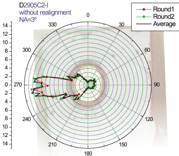
FIG. 4 (color online). Average (far field) emission pattern measured from the microlaser with the same boundary as in Fig. 3. Filled circles mark data points; the lines are guides to the eye. Between measuring *round one* and *round two*, 1.5 hours passed, but all parameters were kept constant. The difference in the signal is due to mechanical imperfections of the setup and a temperature drift.
