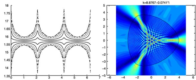
FIG. 2 (color online). Constant width curve. Magnified phase space near the middle line and a quasibound mode concentrated near the caustic. Quasibound mode is a solution of the Helmholtz equation  $\Delta u + k^2 n^2 u = 0$  with  $n = 3.5$  inside the cavity and  $n = 1$  outside of the cavity.
