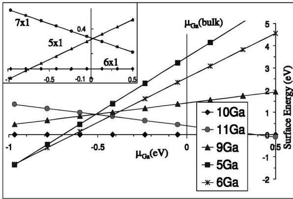
FIG. 3. Surface energy as a function of  $\mu_{\text{Ga}}$  for the most promising Si(112)6  $\times$  1-Ga candidate structures. The structure with 10 Ga atoms per 6  $\times$  1 unit cell (see Fig. 4) is used as reference. Inset: analysis of the stability of the zigzag structure (Fig. 4) with respect to the longitudinal periodicity. Note the different vertical scale (also in eV).
