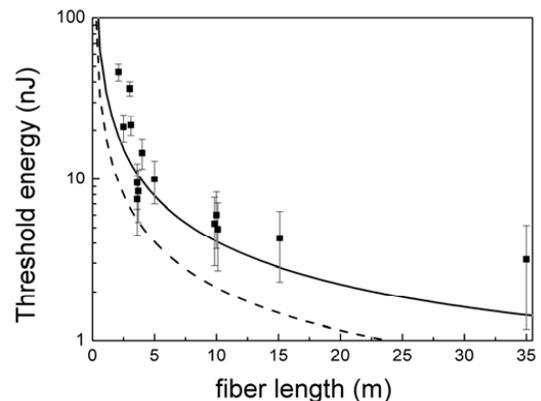
FIG. 3. The evolution of the threshold energy with the fiber length. The points are experimental measurements. The lines are from theory for  $g = 1.5 \text{ cm/GW}$  (solid line) and  $g = 2.68 \text{ cm/GW}$  (dashed line), taken from Refs. [4,11,12], respectively.
