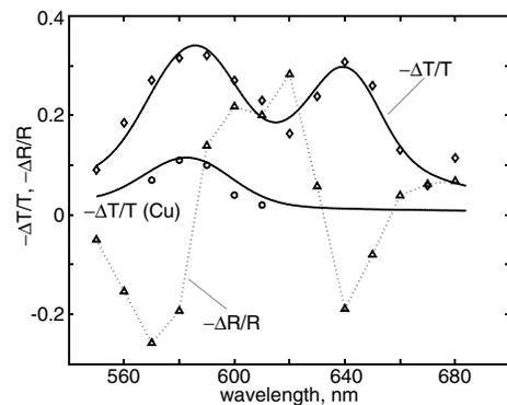
FIG. 4. Measured nonlinear fractional change in transmission (diamonds) and reflectivity (triangles) as functions of wavelength for the MDPC sample. The fractional change in transmission of the bulk Cu (circles) is shown for comparison. The intensity at the focus was  $200 \text{ MW/cm}^2$ . The solid lines represent the phenomenological model described in the text. Note the minus sign on the vertical axis; the transmission decreases with intensity.
