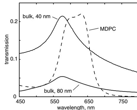
FIG. 1. Measured transmission spectra of the 40 and 80 nm thick bulk copper samples and the metal-dielectric photonic-crystal (MDPC) sample.
