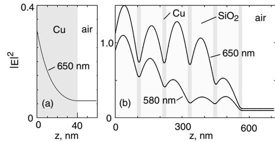
FIG. 2. Numerically calculated  $E$ -field distribution within the bulk 40 nm sample at 650 nm (a) and the MDPC sample at a wavelength of 580 nm (out of resonance) and 650 nm (in resonance) (b). The field distribution is normalized to the incident field.
