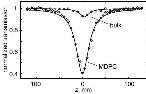
FIG. 3. Z-scan traces showing the normalized transmission of the bulk (circles) and MDPC (diamonds) samples at  $\lambda = 650$  nm as a function of the distance from the focal point. The intensity at the focus was  $500 \text{ MW/cm}^2$ . The solid lines represent the fit obtained by numerical calculations.
