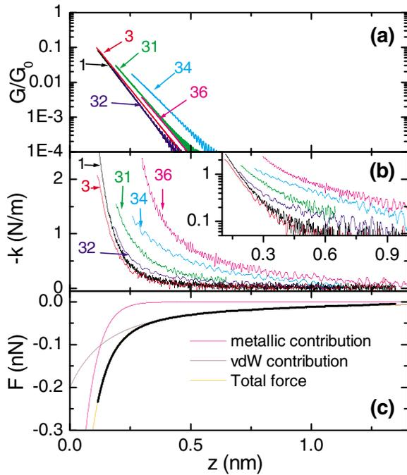
FIG. 2 (color online). (a) and (b) Semilogarithmic plot of the conductance and stiffness of various junction realizations (data sets # 1, 3, 31, 32, 34, 36 in Table I) as a function of the corrected distance axis (see text). (c) Forces obtained by integrating the stiffness for data set #1 showing the vdW and metallic contributions.
