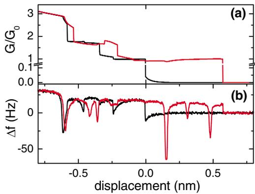
FIG. 4 (color online). Simultaneous (a) conductance and (b) frequency shift measurements for a larger indentation resulting in atomic chain formation.
