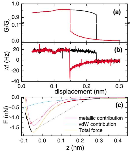
FIG. 3 (color online). Simultaneous (a) conductance and (b) frequency shift measurements for a one-atom junction. (c) Force, with vdW and metallic force components.
