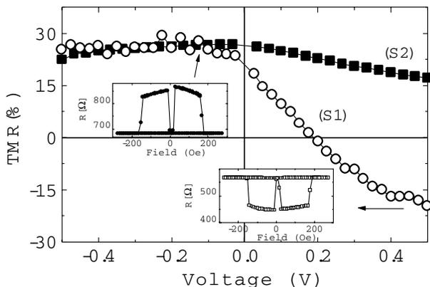
FIG. 2. TMR versus the voltage  $V$  curves measured in samples (S1) and (S2), respectively. Insets: Positive TMR versus magnetic field  $H$  [TMR( $H$ )] curve measured at  $V = -0.1$  V ( $V+$  = top MTJ electrode); negative TMR( $H$ ) curve measured at  $V = +0.5$  V ( $V+$  = bottom MTJ electrode).
