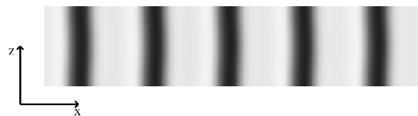
FIG. 4. A chemical pattern moving with the speed of the average fluid velocity \bar{V} = 200 . The width of the rectangular tube is 0.1, while its length is equal to 20.
