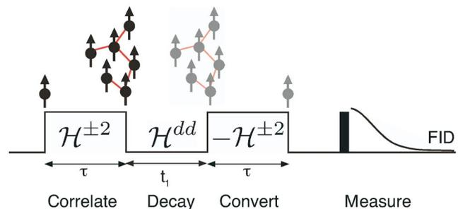
FIG. 1 (color online). Experimental scheme: The effective Hamiltonian  $\mathcal{H}^{\pm 2}$  creates correlations between the spin qubits. During  $t_1$ , these coherences decay. The conversion step transfers the coherence amplitudes into observable magnetization, and the readout measures them as the amplitude of the FID.
