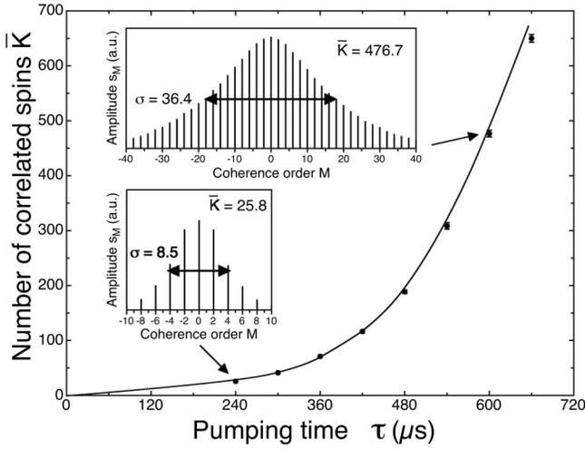
FIG. 3. Size  $\bar{K}$  of the effective quantum register as a function of the pumping time  $\tau$ . The points represent experimental values; the solid line is a guide to the eye. The two insets show examples of the distribution of signal into different coherence orders with half-width  $\sigma$ .
