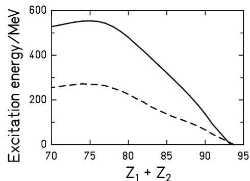
FIG. 3. Calculated mean excitation energies of the prefragment right before entering the ablation stage (solid line) and at the fission barrier (dashed line) for the reaction  $^{238}\text{U}(1 \text{ A GeV})$  on  $(\text{CH}_2)_n$  as a function of  $Z_1 + Z_2$ . The dashed line has been obtained using the description of Ref. [26] with  $\beta = 2 \times 10^{21} \text{ s}^{-1}$ .
