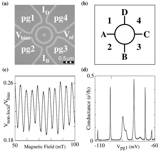
FIG. 1. (a) AFM micrograph of the ring structure. Bright oxide lines fabricated by AFM lithography lead to insulating barriers in the 2DEG. (b) Schematic arrangement of the four terminal ring. (c) AB oscillations in  $V_{nl}$ . (d) Conductance through a quantum dot induced in segment 1 as a function of  $V_{pg1}$ .
