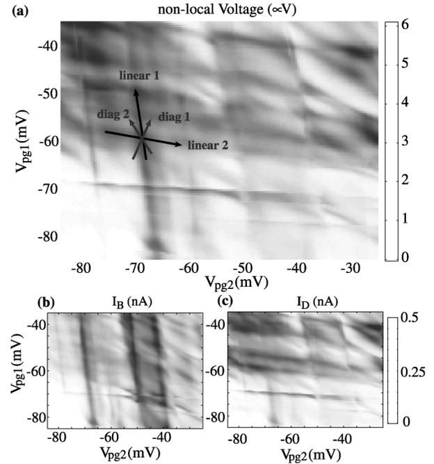
FIG. 2. Plots of (a) the nonlocal voltage  $V_{nl}$ , (b) the currents  $I_B$  and (c)  $I_D$  as functions, respectively, of  $V_{pg1}$  and  $V_{pg2}$  tuning the dots in segments 1 and 2.
