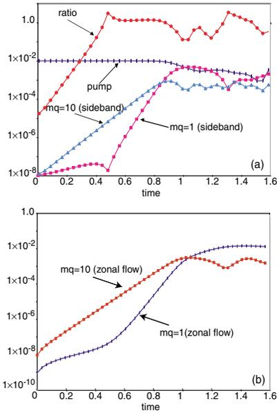
FIG. 2 (color online). Time development of (a) the pump amplitude, upper sidebands with  $m_q = 1, 10$ , and ratio of amplitudes; (b) zonal flow amplitudes for  $m_q = 1, 10$ .
