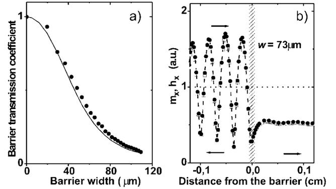
FIG. 4. (a) Barrier transmission coefficient as a function of the barrier width. Full circles: experimental values. Solid line: results of the numerical simulations using Eq. (5). (b) Profiles of the dynamic magnetization,  $m_x$ , (full circles) and dipole field,  $h_x$ , (open squares) in the wave, normalized to the values of the incident wave. The dashed line is a guide to the eye. Incident, reflected, and tunnelled waves are indicated by the arrows. The barrier is shown by the hatched area.
