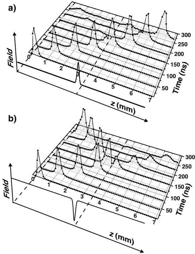
FIG. 3. Propagation of a spin-wave packet across a YIG film with local field inhomogeneity, observed by space- and time-resolved BLS. (a) Field/gap has a local maximum, creating a potential dip for the wave; (b) field/gap has a local minimum, creating a potential barrier for the wave. The maximum absolute value of  $H_j$  is the same for both cases and is 56 Oe. An animated version of this figure can be viewed in the online/PDF version of this Letter.
