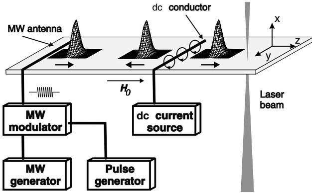
FIG. 1. Schematic layout of the Brillouin light scattering setup in the forward scattering geometry with space and time resolution for the study of spin-wave propagation through an inhomogeneous magnetic field. For a discussion of the components, see the main text.
