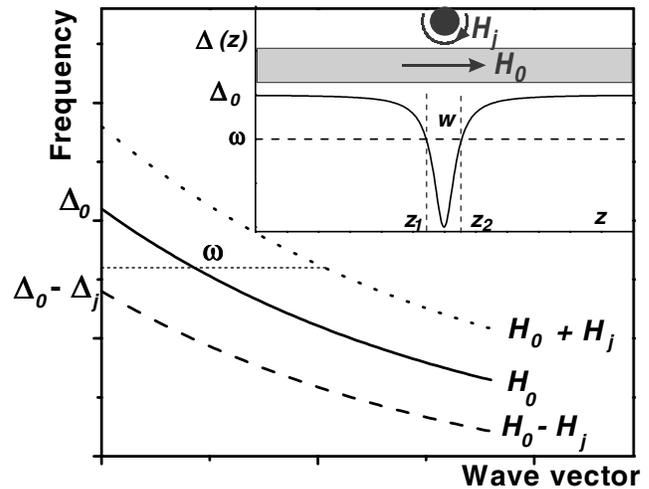
FIG. 2. Spectrum of BVMSW in a magnetic film.  $\Delta(z)$  is the gap of the spectrum. The inset illustrates the profile of the gap, the creation of the turning points, and the forbidden interval due to the inhomogeneous field, caused by the dc conductor.
